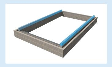
**4** To start, insert the 1200mm long narrow infill blocks (Noted as 'N' on the layout drawings). **Note:** To ensure all offcuts are usable within the floor layout, end panels should not be cut less than 300mm or over 900mm.
