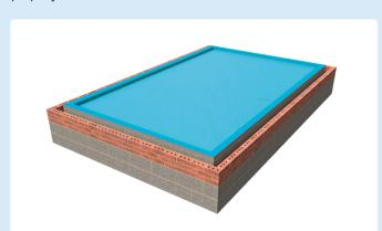
**8** Place the 80mm or 150mm thick top sheet over the floor. At the end of the first row cut the top sheet to suit and start the second row with the offcut.
