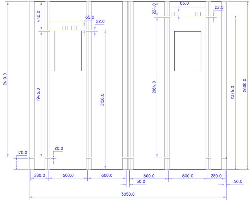
Front Elevation - Secondary Steel Layout
