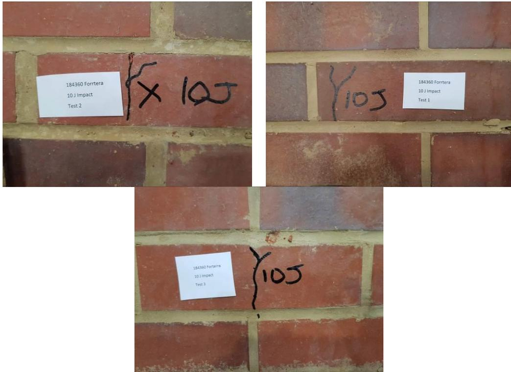
**Plate 16 – Dark Multi Smooth Brick Slip Hard Body Impact Tests (10 Joules)**
