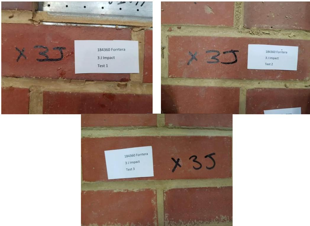
**Plate 18** – Dark Multi Smooth Brick Slip Hard Body Impact Tests (3 Joules)
