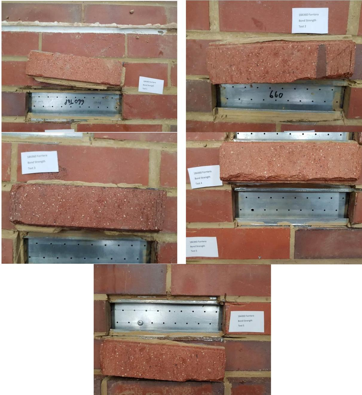
**Plate 21 – Dark Multi Smooth Brick Slips Bond Strength Tests – after Hygrothermal, Freeze/Thaw Testing and Water-Tightness Testing**
