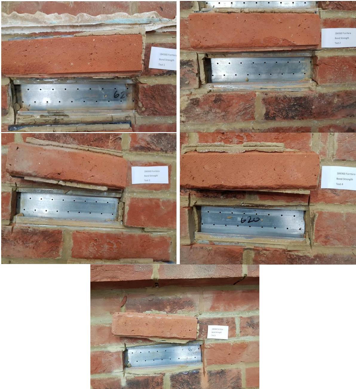
**Plate 22** – Chelsea Smoked Red Brick Slips Bond Strength Tests – after Hygrothermal, Freeze/Thaw Testing and Water-Tightness Testing
