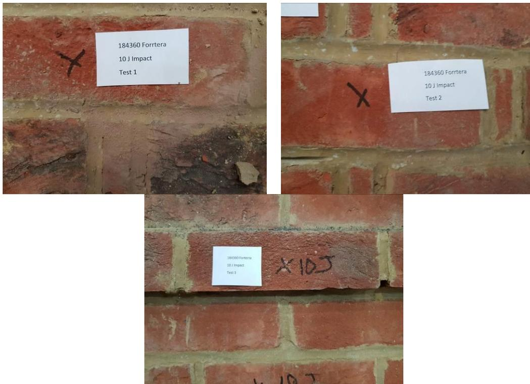
**Plate 17 – Chelsea Smoked Red Brick Slip Hard Body Impact Tests (10 Joules)**
