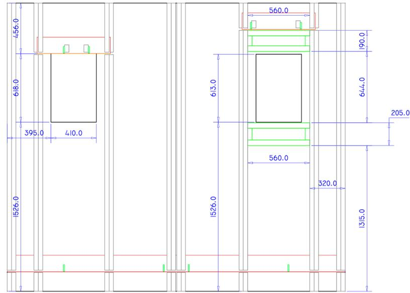
Front Elevation - Timber Batten, DPC & Perpend Vent / Drain Layout
