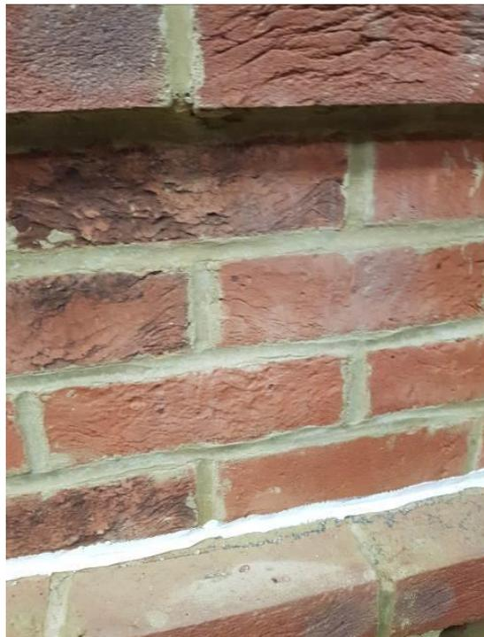
**Plate 20** – Soft Body Impact Test Chelsea Smoked Red Brick Slip 400 Joules – No Damage
