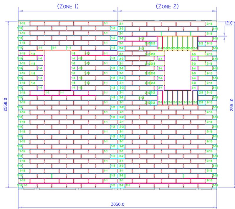
Front Elevation - Brickwork Layout
