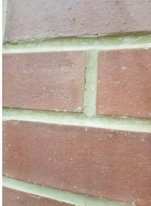
**Plate 19** – Soft Body Dark Multi Smooth Brick Slip 400 Joules – No Damage
