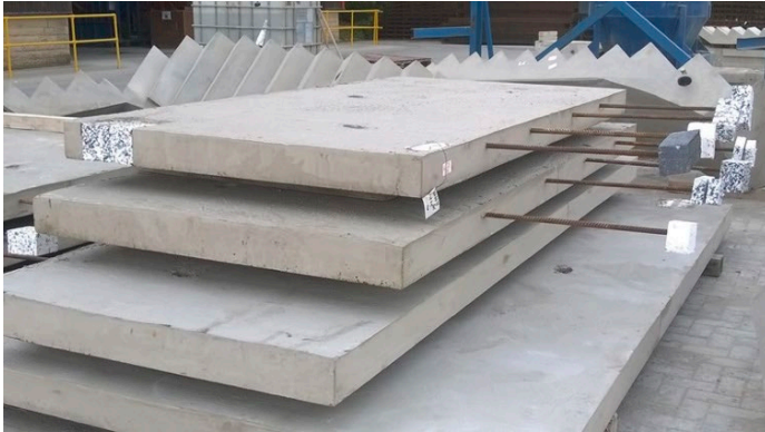
Figure 10 – Simple RC slab with cast in bars for tying back to the main floor slab.
