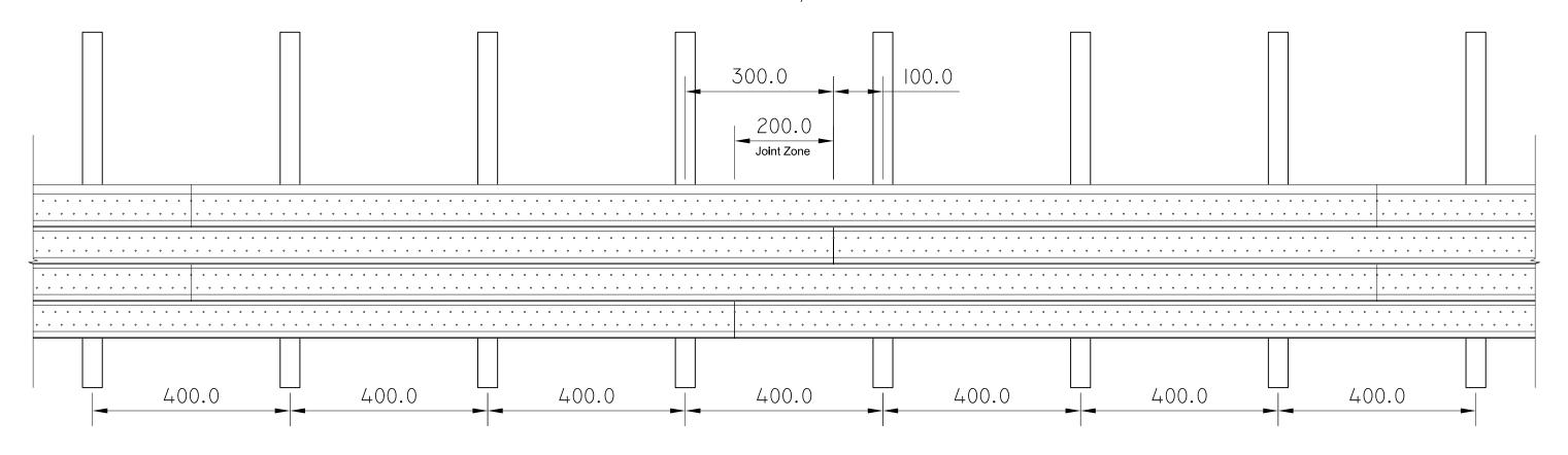
No two (vertical) joints in adjacent rails in the same bay. Joints between rails in the course above or below must be in another bay.
