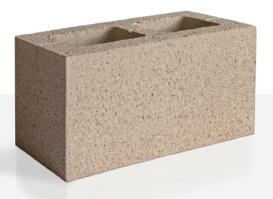
This block is manufactured with full height voids which reduce the unit's overall weight. Steel reinforcement can be located in the block voids which is then surrounded with suitable poured concrete to created reinforced structures.
